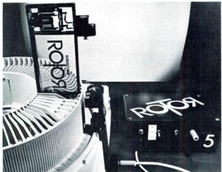
The Rotor device atop the drum with the drum-attached interface unit and the control box.
