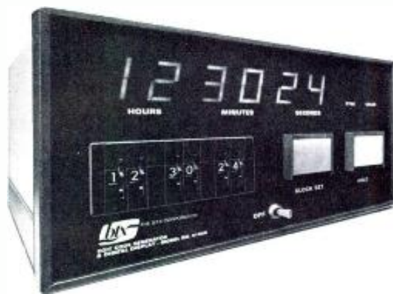
Figure 3. The BTX Model 4100A SMPTE code generator is used to lay down a code track on audio or video tapes.
