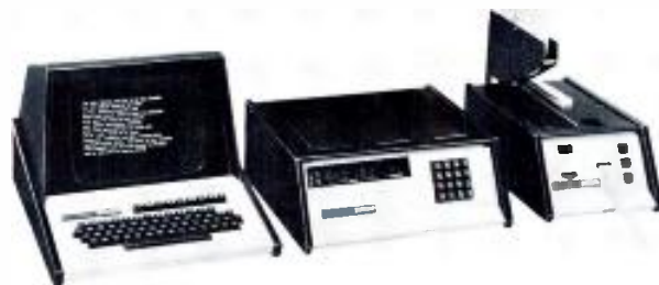
A typical Heathkit H-8 system with the H9 video terminal and H10 papertape reader/punch. Not shown, a standard cassette unit can be used instead of the papertape unit.
