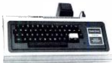
The basic Radio Shack keyboard/CPU system with the power supply shown behind. Expander units are available to increase capacity.
