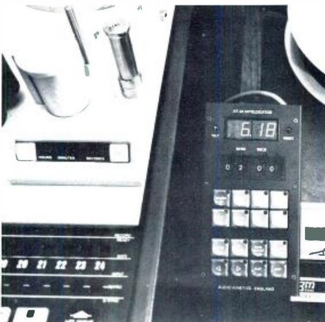
On the left, Ampex' Search-To-Cue and tape timing accessory. Next to it is the Audio Kinetics XT-24 Intelocator, which may be interlaced with Ampex, 3M, or other machines.
