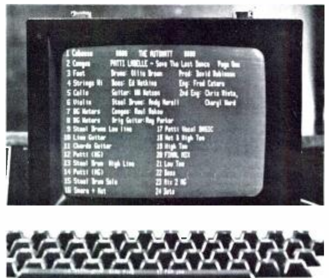
Figure 3. This interface of systems is capable of storing any desired text along with the console automation data on the tape. Automatically recalled the text pictured includes information regarding track assignments, musicians, artist's name, title of song, and recording personnel.
